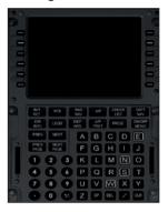
When loading the aircraft, the CDU will be in a 'Cold & Dark' state. Press the **ON/OFF MENU** button to switch on the CDU unit.
