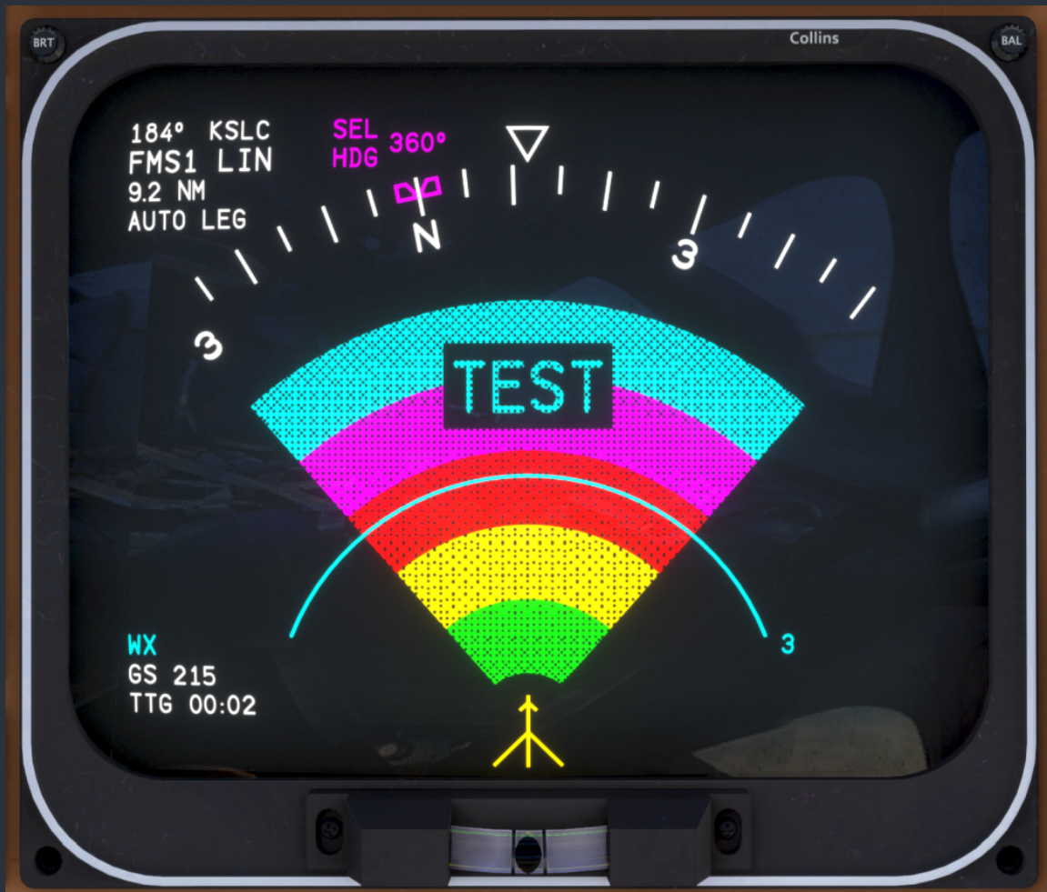
Radar test pattern on ND ARC display
