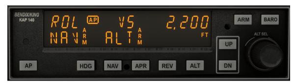
The UP/DN buttons are used when setting your vertical speed while in VS mode and the inner/outer dial is used for setting the Altitude Reference.
