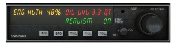
This convenient maintenance and status screen uses standard green, yellow and red letters to show severity levels of each area. Engine health is a very long running failure of 300 – 500 hours, however excessive abuse can shorten the engines lifespan. Being fouled, running with low oil, and even over revving can have a detrimental effect.
