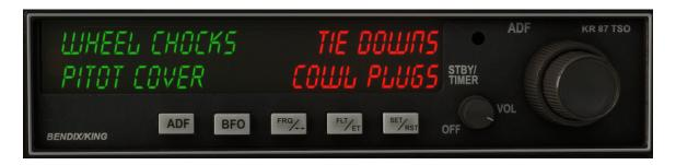
The selection of the external elements can be done here. Red means that that element is in place. Anything left on will have an impact on your flight. From not being able to taxi because you're tied down, to overheating the engine because you took off with the cowl plugs still in.
