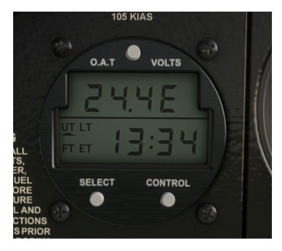
You will notice the 4 timer functions in the lower left of the display. These have been modified to work according to the Davtron 803 Clock Operation Manual, including a FT alarm, an ET countdown mode with alarm, FT reset, and screen test. The ability to also set LT to 12 or 24 hour formats is also included, and is done by holding down the CONTROL button for 3 seconds while in LT mode.
