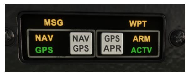
You can see the two push buttons that work with your autopilot and the GNS systems. The GPS APR button will activate the loaded approach.
