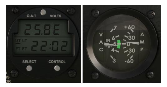
Press the top button to toggle between Outside Air Temperature and battery voltage
