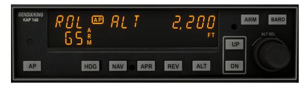
Here, the APR button has been pressed as indicated by the GS ARM mode in the lower left of this display. This AP unit connects to the GNS 530/430 flight plan and changes their screens from GPS mode to VLOC mode for you.
