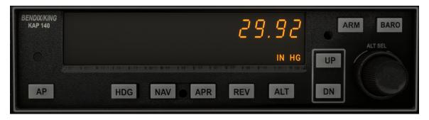
When you first power up your plane, the standard pressure (North America) is flashing on this unit until you press the BARO button. If you long-press the BARO button, it will change to HPA. Use the inner/outer dial to set the barometric pressure here anytime you adjust it on your Altimeter.
