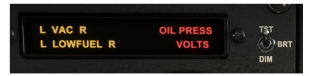
The switch works as it should with the TST (test) to show all lights are working and the bright/dim functionality that is needed in day or night flight. The test function purpose is to ensure all the light bulbs behind that screen work properly before flight. (similar to turning the key in your car and seeing the dashboard light up before you start the engine)
