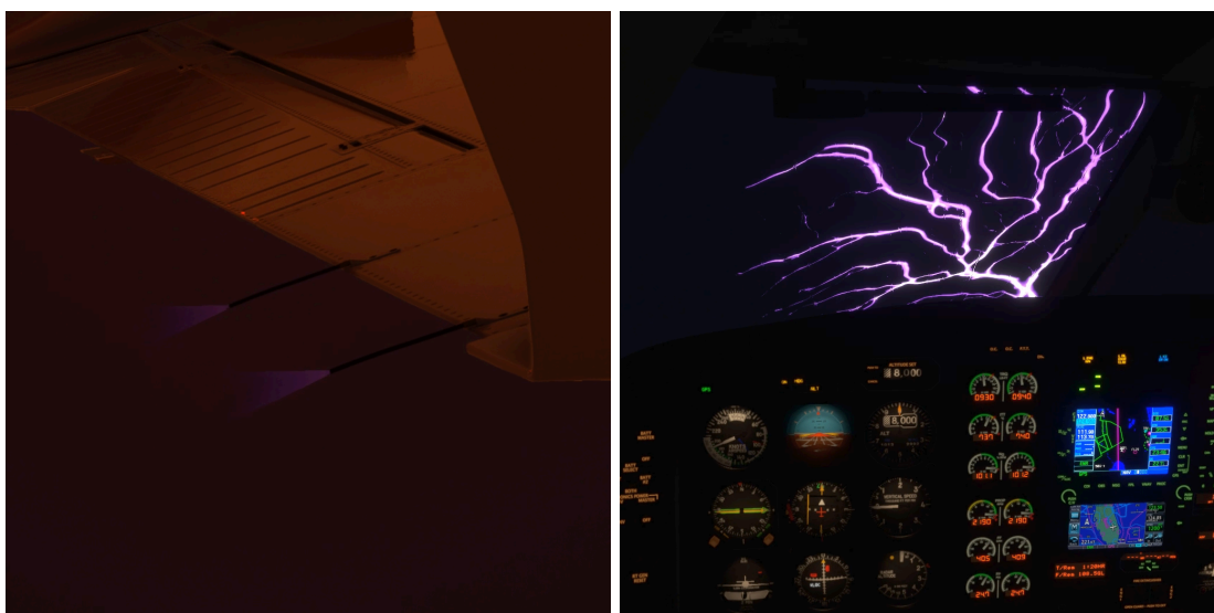
Corona Discharge (St. Elmo's Fire), and Electrostatic Discharge
