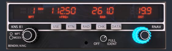
3. Once our desired frequency has been set we will use the "DATA" push button to page through the three required pieces of data in this data channel in the order "FREQ", "RAD", and "DST". Press the "DATA" button once, and then enter the radial 154.0, again with the dual concentric rotary knobs. Should your desired radial include a decimal component, the inner rotary knob can be pulled and rotated for decimal entry.
