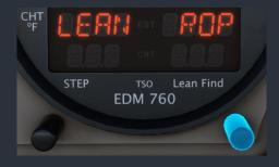
Both methods of leaning begin by "pre-leaning" the engine to approximately 50°F (28°C) EGT rich of peak on any cylinder. After waiting for temperatures to stabilize, begin leaning the engine. When a dot begins flashing above one of the cylinder columns to indicate the hottest cylinder, Lean Find mode is now armed, and an approximately 15°F (8°C) increase of average EGT has been observed.
