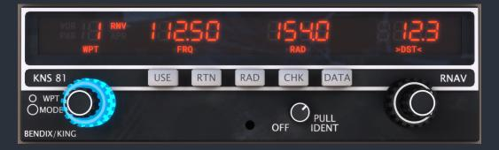
NOTE: VOR modes of operation WILL NOT provide CDI or DME information relative to the active waypoint. They are for operation as a conventional navigation radio with reference to existing VOR stations, in either angular or linear course deviation mode.
