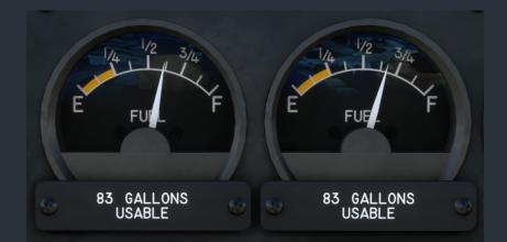
NOTE: Conventional fuel sender units in aircraft are notoriously sensitive to lateral G-force, and how level the aircraft is sitting on the ground. The fuel quantity gauges may appear to indicate incorrectly, as a result, though this is accurate to the real aircraft. Given that this aircraft is also capable of random fuel leaks, fuel levels should be checked prior to takeoff, just as in the real aircraft, when any potential discrepancy exists.
