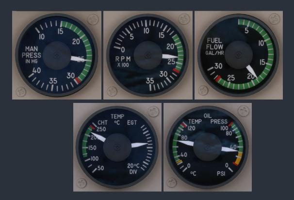
The pressurized version of this aircraft is equipped with different engines than the normally aspirated version, as well as turbochargers. The turbocharged engines are capable of operating at wide-open throttle manifold pressures of up to 39.5 inHg, and fuel flows that may approach 40 GPH.
