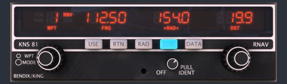
4. When our desired radial is set, press the "DATA" push button once again to enter our desired distance offset of 12.3 nm. Again, should your desired distance include a decimal component, the inner rotary knob can be pulled and rotated for decimal entry.
